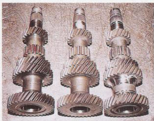
These three laygear assemblies incorporate various BGH mods. On the left is the assembly from a standard 2-litre gearbox, modified to accept a heavy duty roller bearing and incorporating a long (high) ratio first gear — 18 teeth running with 34. In the centre is a 2.8-litre V6 type laygear, also accepting the heavy duty roller bearing and with a long first gear ratio — 19 teeth running with 33. On the right is a modified laygear with close-ratio gears, and designed for the heavy duty roller bearing. A long first gear ratio is used, and the gearset closes the normal gap between second and third ratios, providing the ultimate gearing for track day and road use.
