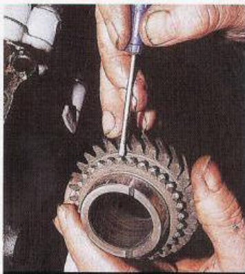
Closely examine the condition of all the dog teeth throughout the unit. Look for clear-cut profiles — rounded/broken edges indicate wear/abuse.
