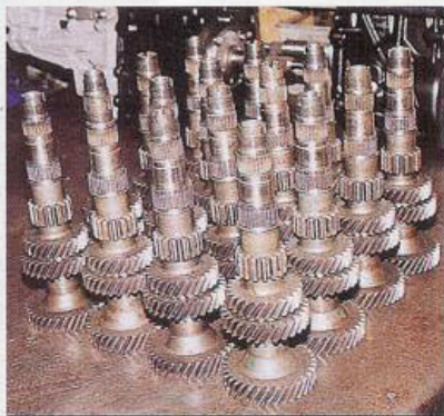
BGH keep in stock a huge range of components for the Type-9 units. This is a small selection of standard 2-litre laygears, incorporating long (high) first gear ratios, as modified by Brian.
