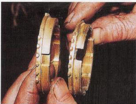
A sign of trouble is breakage of the edges of the hub plates (inserts). The sheared edges can dig into the baulk ring, so that the insert cannot slide out of engagement as designed. It can then be difficult/impossible to take the car out of gear.
