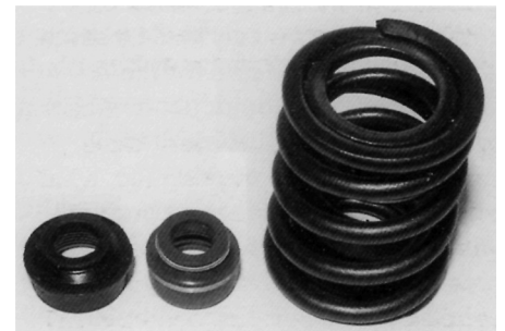
Standard valve stem seal (left) and smaller diameter oil seal which will fit inside dual valve springs (right).
