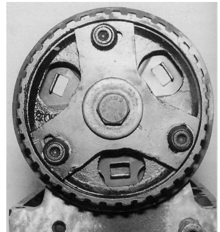
Adjustable ('vernier') camshaft sprocket/wheel.
