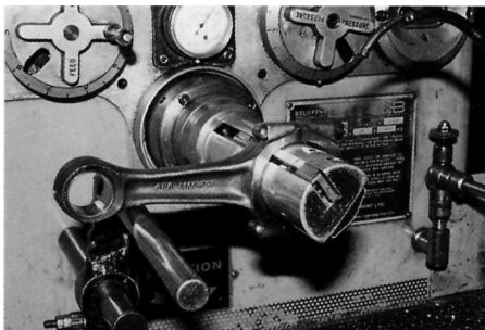
Connecting rod bearing tunnel being honed.
