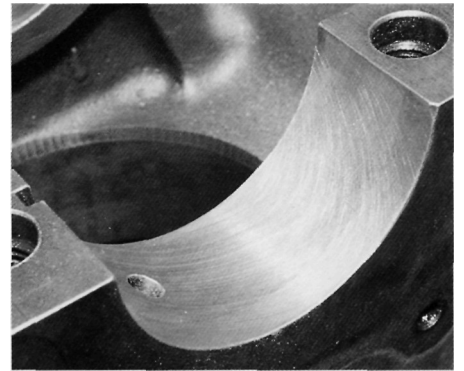
Main bearing tunnel bore surface as machined by the FoMoCo. Nothing less than this finish will do.
