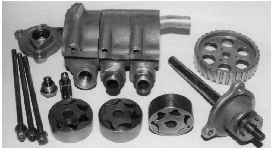
Components of a dry sump pump appropriate for Pinto/Cosworth.
