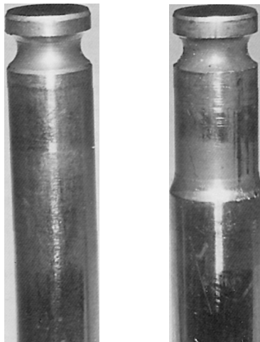
Valve stem keeper groove detail.
