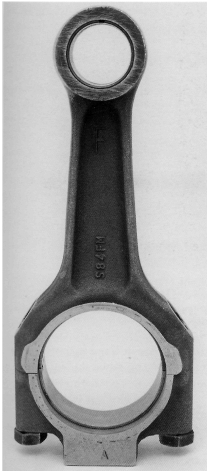
1600cc Ford diesel connecting rod (small end has been lightened).
