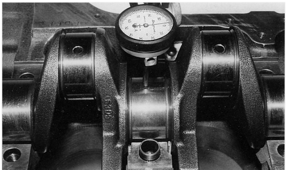
Measuring crankshaft runout (straightness).
