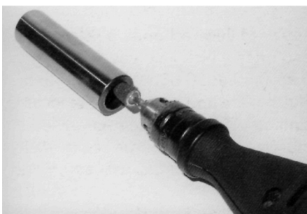
Piston pin having material removed from the inside using a high-speed grinder fitted with a mounted point grinding wheel. Up to 5 grams can be removed easily using this method without detriment to the strength of the piston pin.
