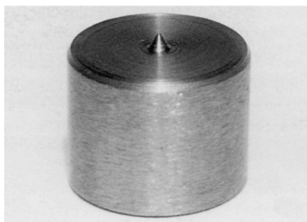
The special spotting punch made to mark the back of the flywheel - the punch must be hardened.
