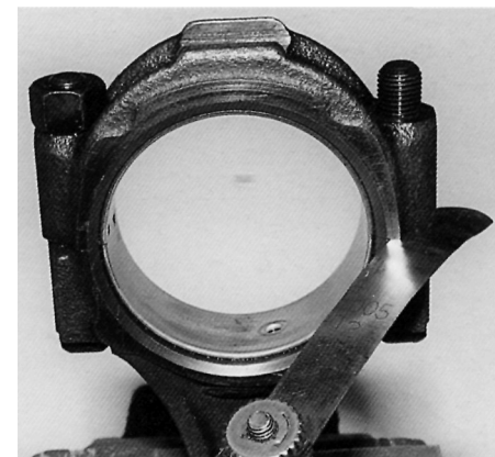
Cap 'sprung' by bearing crush. Feeler gauges inserted between the cap and rod should reveal a 0.1-0.15mm/0.004-0.006in gap.
