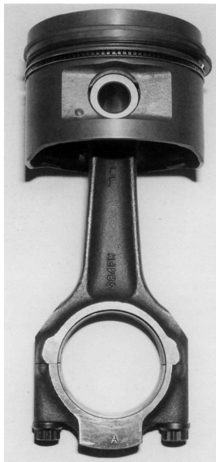
Kolbenschmidt piston and Fiesta 1600 diesel connecting rod assembly, note the Cosworth connecting rod bolts (a good move).
