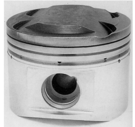
Raised top, 12 to 1 piston for a naturally aspirated Cosworth engine.
