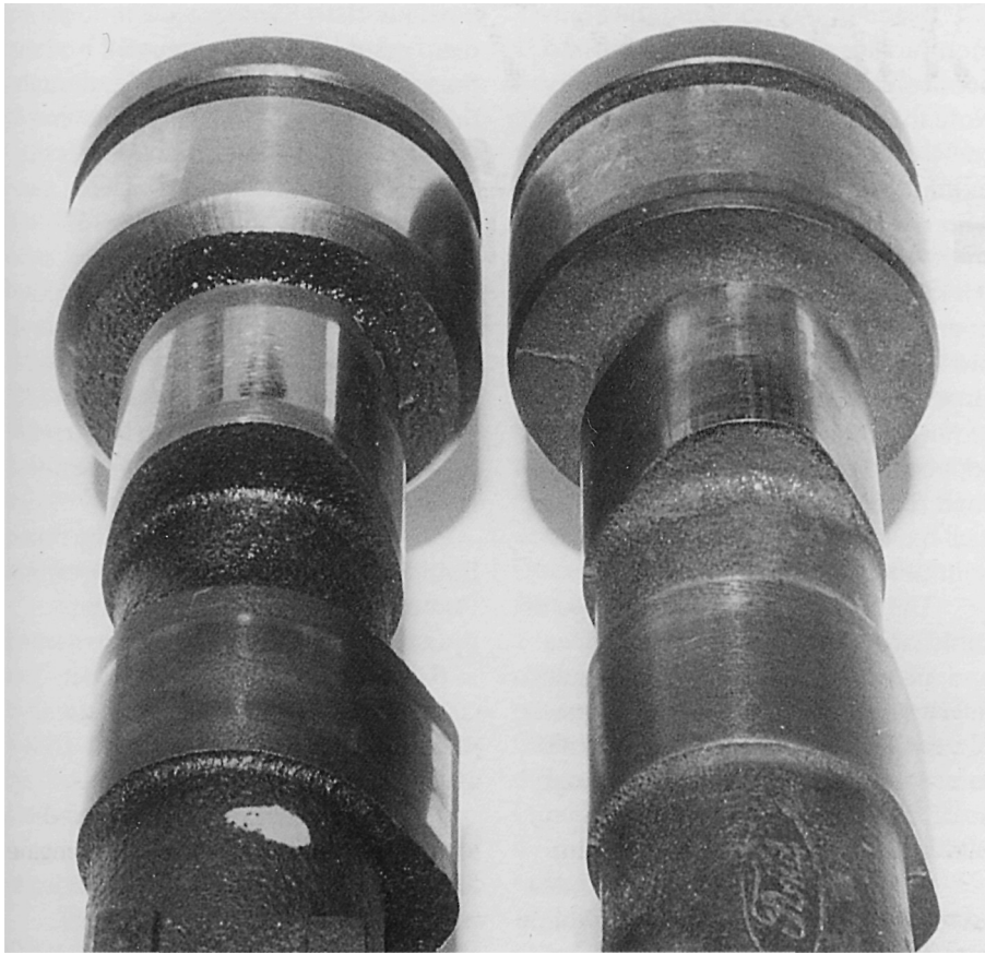
Standard camshaft on the right and a performance camshaft on the left. Core diameter is smaller on the performance camshaft and so is the base circle. The toe of the camshaft lobe on each camshaft is in the same place (approximately) in relation to the camshaft axis.
