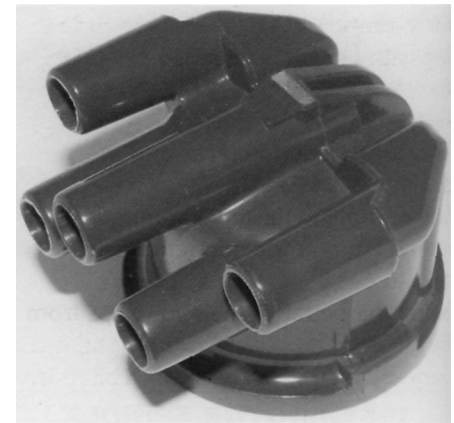
Distributor cap with horizontal HT terminals. Ideal for carburetted Pintos.
