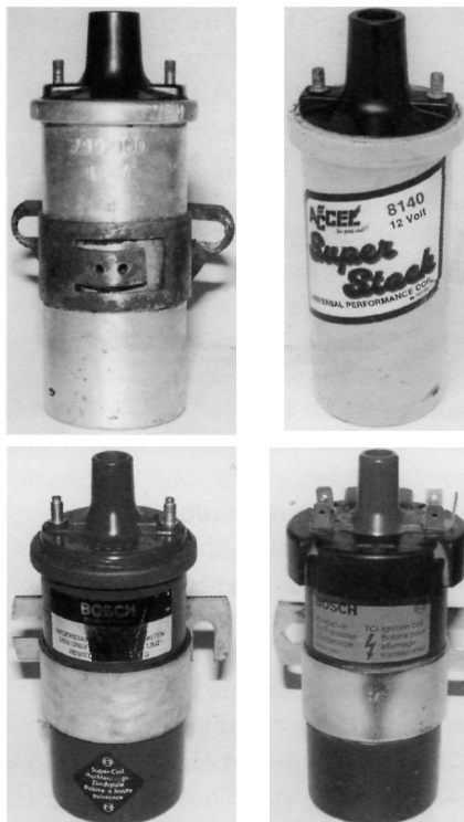
Clockwise from top left - standard conventional coil; typical uprated coil (approx. 28Kv); typical ballast resistor coil; typical oil-filled 'electronic' coil (up to 37Kv).
