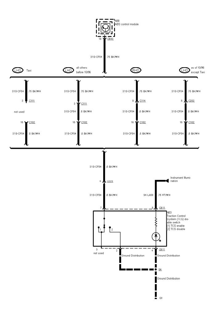
12-02-007 , ABS with Traction Control System (TCS) , Except 2,9 I V6 12V
