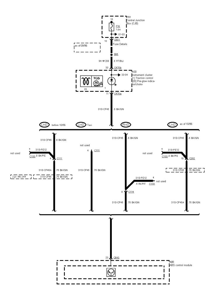
12-02-005, ABS with Traction Control System (TCS)
