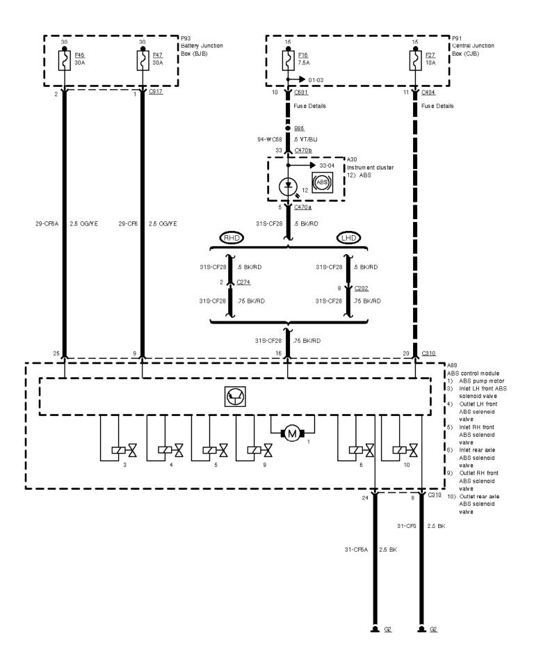
12-03-002 , Anti-lock Braking System (ABS) MK 20-I
