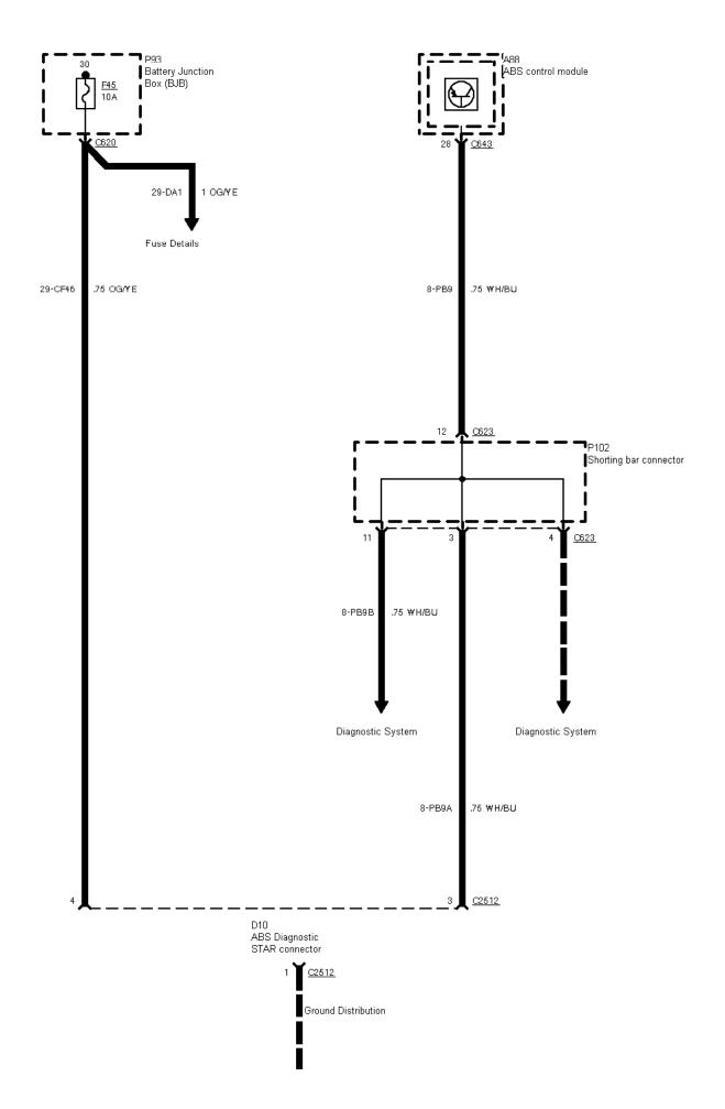
12-02-011 , ABS with Traction Control System (TCS) , Diagnostic connectors
