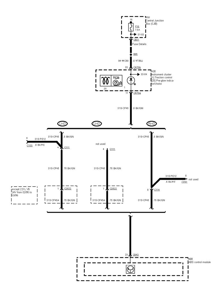
12-02-004 , ABS with Traction Control System (TCS) , as of 03/96
