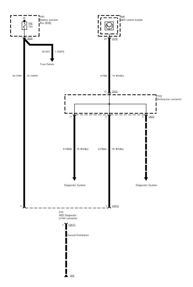
12-03-004 , Anti-lock Braking System (ABS) MK 20-I , Diagnostic connectors
