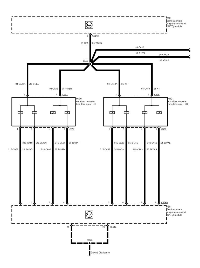
${\bf 34\text{-}04\text{-}004}$  , Air Conditioning with SATC , Door motors
