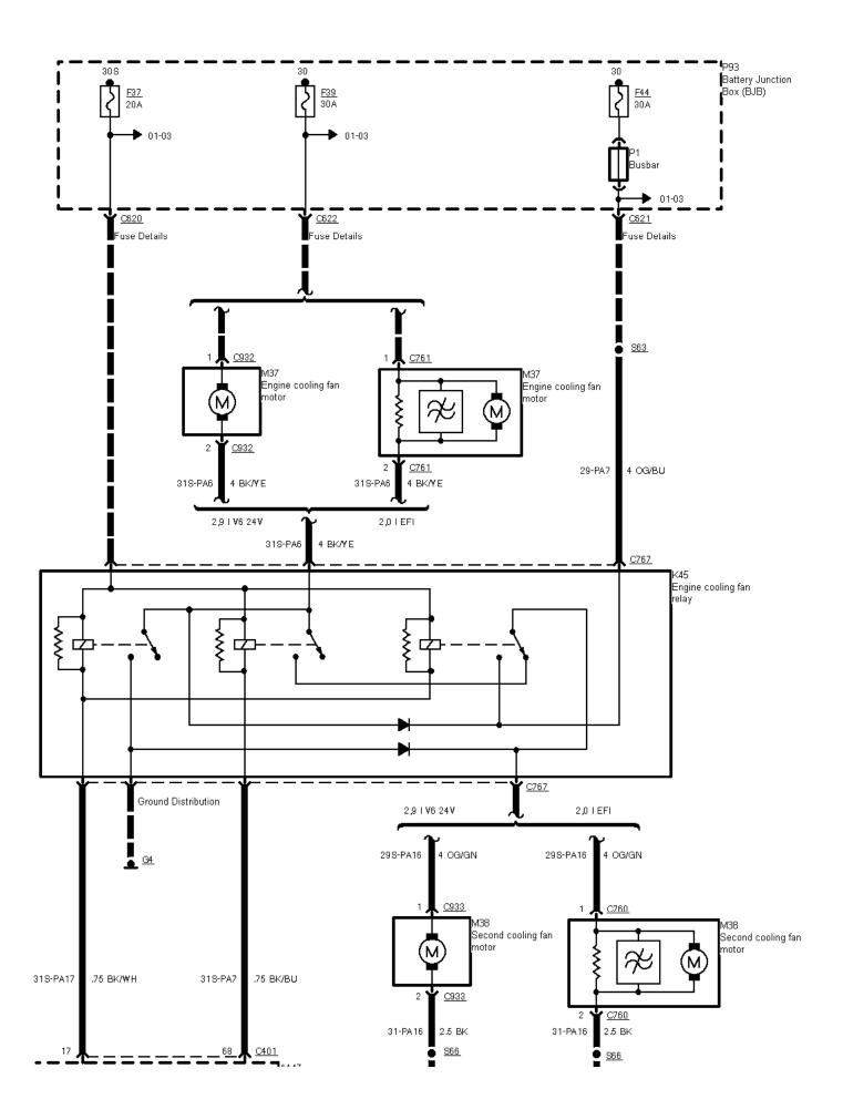
34-04-012 , Air Conditioning with SATC , Engine cooling fan, 2,9 l V6 12V
